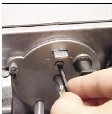
fig. 15 : Combustion head adjuster screw
